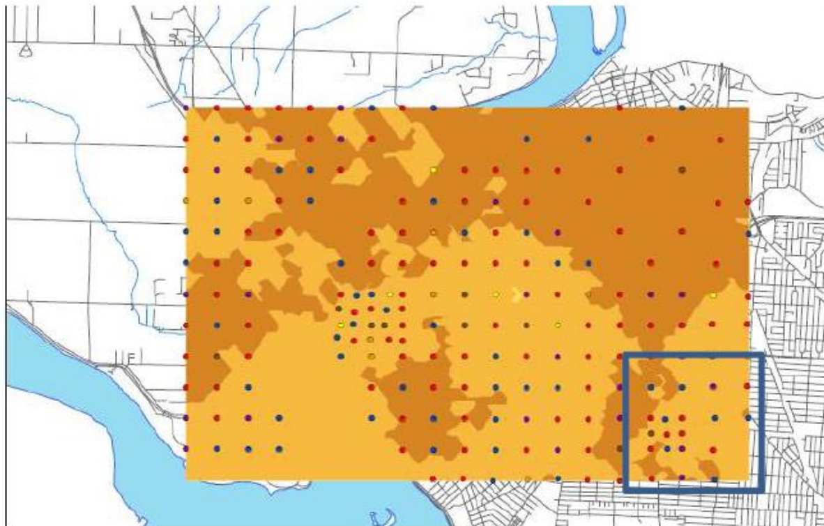
Figure 4 Simulated "Hot Spot" map developed from data from other sites. Data is for polycyclic aromatic hydrocarbons. Elevated regions are shown by darker shade of brown.
